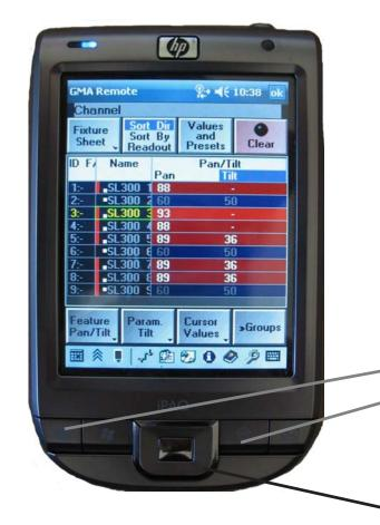
the *grandMA* console will be installed on the PocketPC. The software will recognize the operating systems Pocket pc, Windows Mobile pocketpc 2003, Windows Mobile pocketpc 2003 SE (Second Edition), Windows Mobile 5.0, Windows Mobile 6.0 Classic and will automatically install the respective modules.
