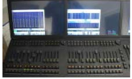
*full-size:* faders 1 - 10 are displayed on the left screen, faders 16 - 25 are displayed on the ecenter screen; faders 11 - 15 and 26 - 28 are not active; faders 29 and 30 work as *Preset- and Executorfader "Set Time / Man Fade"*
